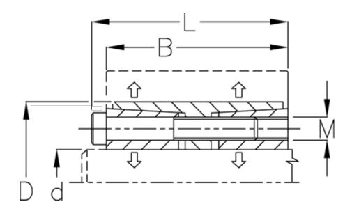
$\begin{array}{lll} \text{B mm} & = 80 \\ \text{d H8 mm} & = 95 \\ \text{D mm} & = 135 \\ \text{Fit tolerance} & = \text{Aksel h8, Nav H8} \\ \text{F kN torque} & = 215.0 \\ \text{L mm} & = 90 \\ \text{M mm} & = \text{M10} \\ \text{P N/mm2 surface pressure on shaft/hub} = 36 \end{array}$
